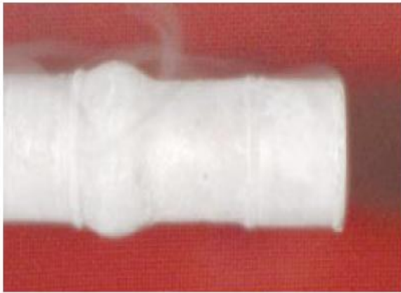
Figure 5: Used to compare the strengths of water ice and methane hydrate, a sample containing both was subjected to axial stress from a piston inside a cryogenic container about 25 millimeters in diameter. Inside this vessel, the weaker water ice (toward left of photo) deforms, causing a bulge, while the stronger methane hydrate under the same stress does not bulge
