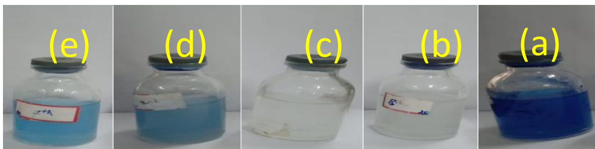
Figure 4: Images of methylene blue solution for (a) no catalyst, (b) 0.5-Cu-TiO 2 , (c) 1.0-Cu-TiO 2 , (d) 2.0-Cu-TiO 2 , (e) 3.0-Cu-TiO 2
